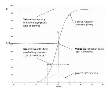
Fig. 1. Schematic diagram of a *simple logistic S-curve*, defined by three parameters: (1) Saturation, (2) Growth time, and (3) Midpoint. The *growth rate function* is represented in scale on the same plot by "bell" shape curve.
