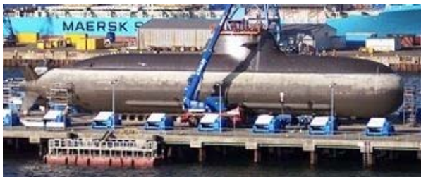
Type 212 submarine with fuel cell propulsion of the German Navy in dock
